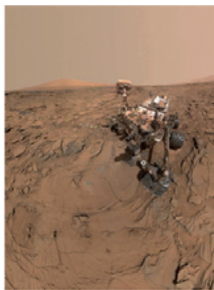
The top of the rover's mast faces away in this May 11, 2016, self-portrait of NASA's Curiosity Mars rover, which shows the vehicle at the "Glorus" drilling site on lower Mount Sharp. The scene is a mosaic of multiple images taken with the arm-mounted Mars Hand Lens Imager (MAHLI). Credits: NASA/JPL-Caltech/MSSS Full image and caption
