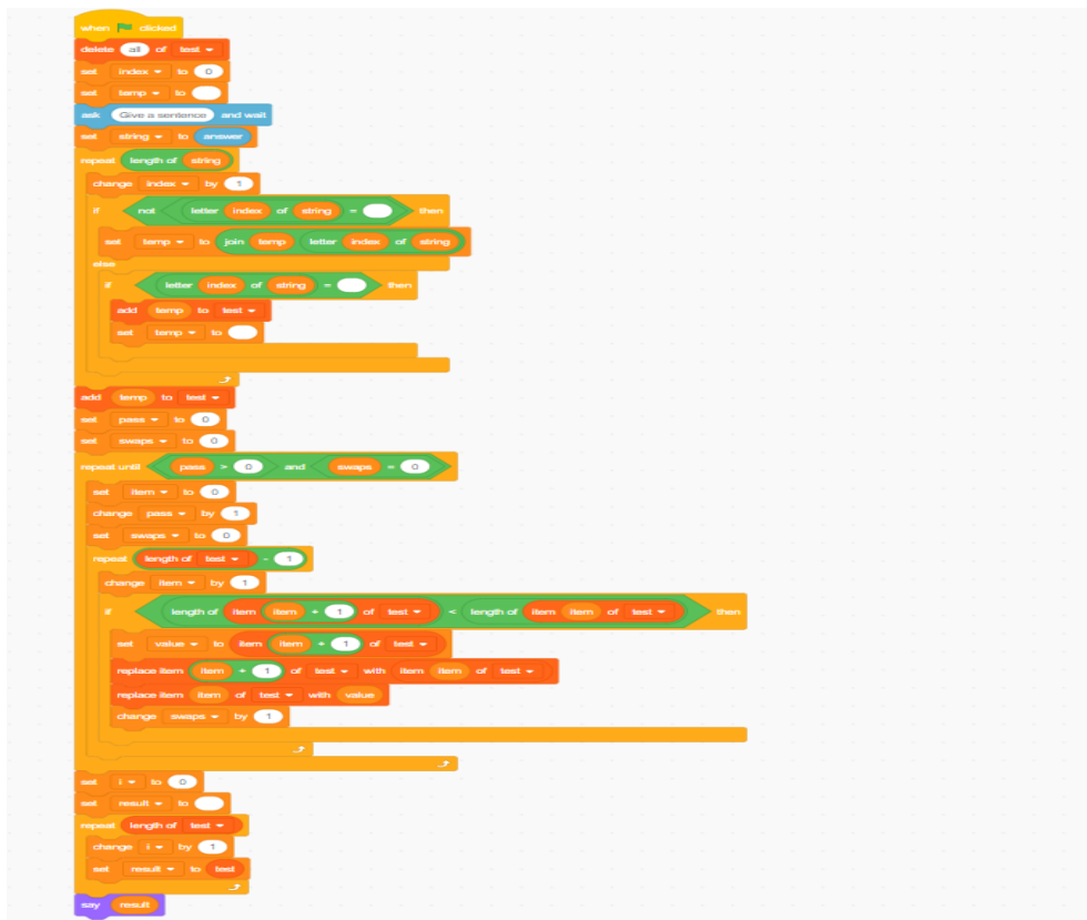
Figure 3. Scratch implementation of a snowball generator: initialisation, user input, and loop-based construction of incrementally longer lines.
