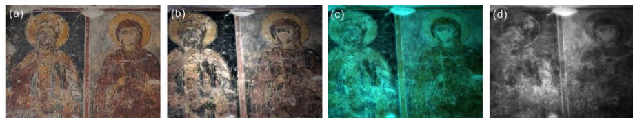
Fig. 5. Multispectral images of the wall painting No. 8: (a) Visible (Vis) image, (b) Mixed Vis and IR images (luminosity), (c) false-colour IR image, (d) UV images.
