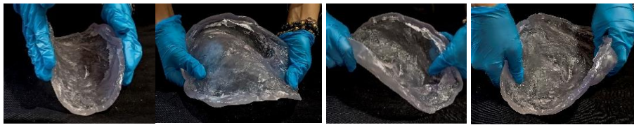
Fig. 5: Elastic deformation of the printed Elastic 50A counterform of element no. 29.
