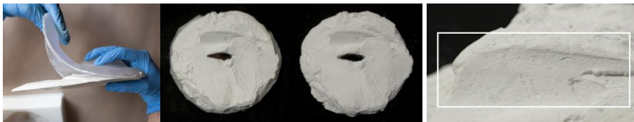
Fig. 6: (from left) Demolding of the positive from the printed Elastic 50A mold; original element No. 29 and exhibition copy comparison; detail of the area characterized by printing layer lines on the copy.
