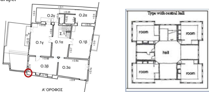
Fig. 6a Repair -reinforcement in SW corner (red cycle) in all floors due to the (arbitrary) placement of a pillar of a neighbor building! 6b The formation of the 1 st floor proves the relation with Ottoman similar layouts.
