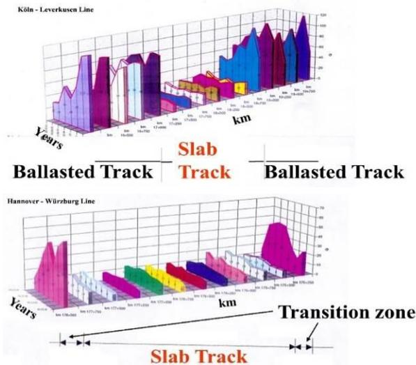
Fig. 5: Quality Index of Slab Track vs Ballasted Track in the Line Köln-Leverkusen (upper illustration) and (lower illustration) in the Line Hannover-Würzburg Germany (Γιαννακός 2012, 2000)
