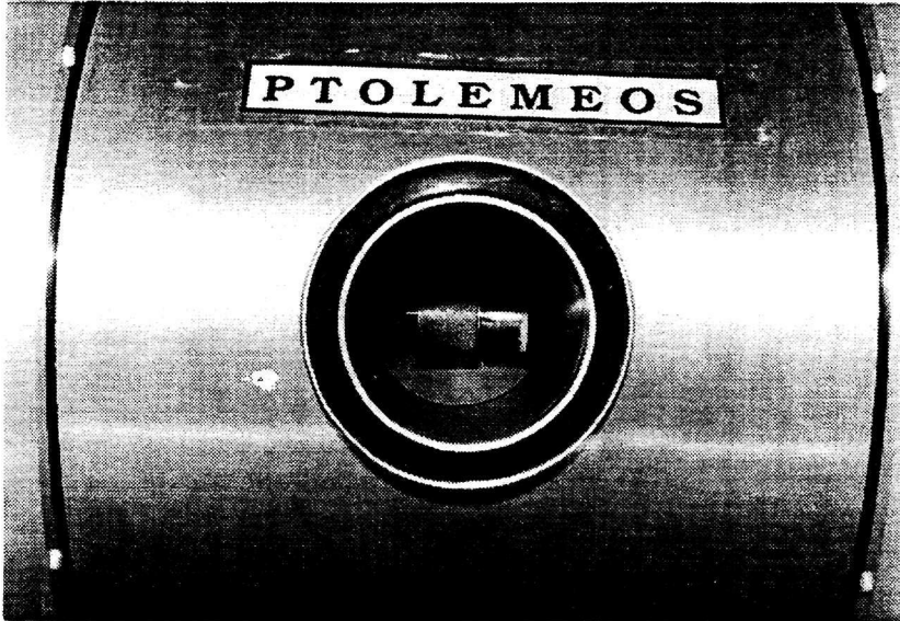
FIG. 11: The target system in the crystal barrel
