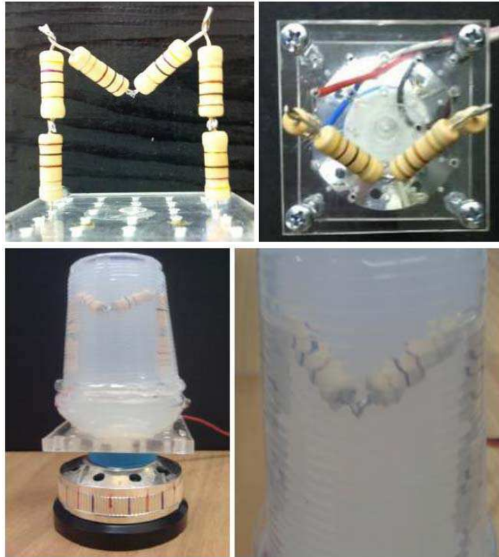
Fig. 2. Upper Part: The thermal phantom used in this study placed on a rotating table. It consists of six resistors connected in series. Phantom dimensions: 50 \text{ mm} \times 50 \text{ mm} \times 15 \text{ mm} . Lower Part: The thermal phantom incased in agarose gel environment (1gr/100ml concentration) Phantom dimensions: 100 \text{ mm} \times 70 \text{ mm} \times 60 \text{ mm} .
