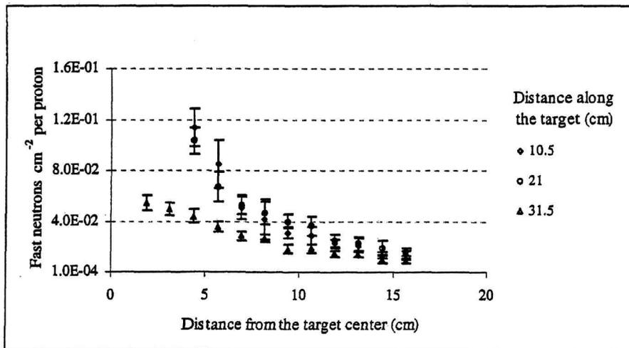
Figure 1. Fast neutron distribution inside target sections
