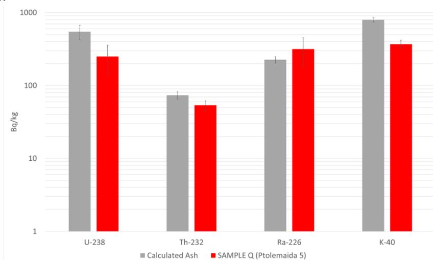
**Figure 5.** Comparison of theoretically calculated concentrations with measured concentrations in bottom ash (sample Q) for the “Ptolemaida 5” CPP. Propagation of uncertainty and coefficient of variance is used for the error-bars of calculated and measured concentration, respectively.
