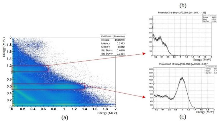
**Figure 4:** 2D coincidence histogram displaying the energy recorded by the plastic scintillator on the x-axis and the energy detected by the CsI scintillator on the y-axis according to the Geant4 simulation(a). On the right, two x-projections are shown: (b) a projection taken outside the coincidence region and (c) a projection within the coincidence region.
