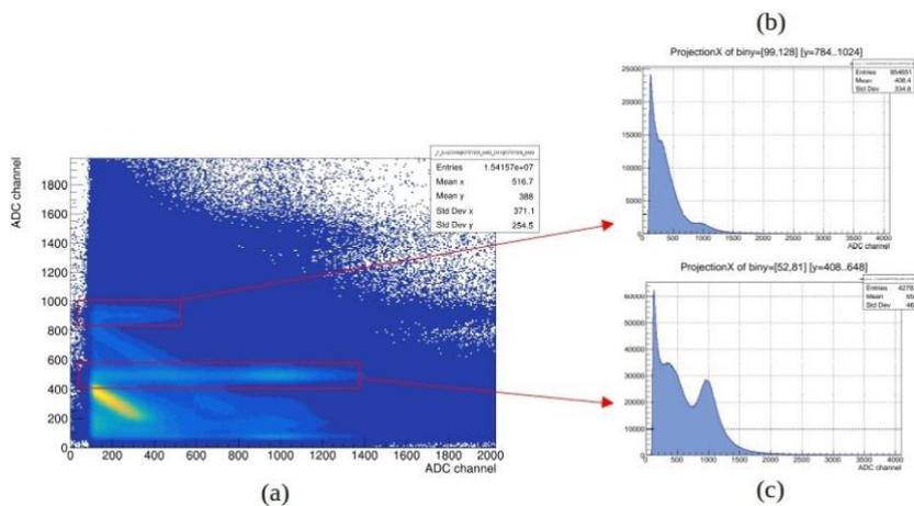
**Figure 3:** 2D coincidence histogram displaying the energy recorded by the plastic scintillator on the x-axis and the energy detected by the CsI scintillator on the y-axis (a). On the right, two x-projections are shown: (b) a projection taken outside the coincidence region and (c) a projection within the coincidence region.
