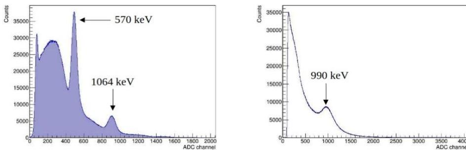
**Figure 2:** Single spectra obtained from a radioactive source of  $^{207}\text{Bi}$  obtained with the CsI scintillator (left panel) and with the plastic scintillator (right panel) The two peaks in the left panel corresponds to the  $\gamma$ -rays of the 570 keV and 1064 keV, respectively.
