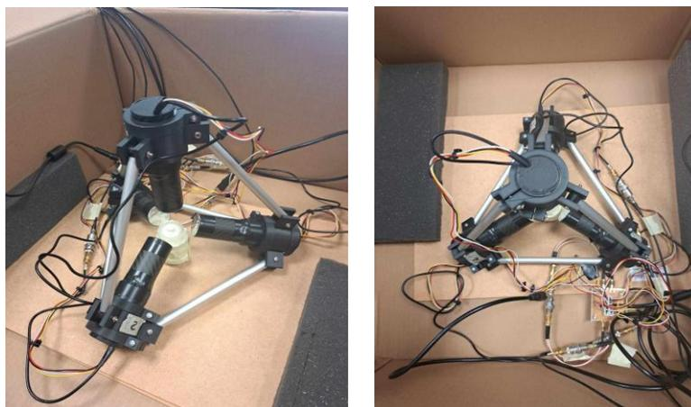
**Figure 2:** A picture of the multi-detector array. Side view (left). Top-down view (right)
