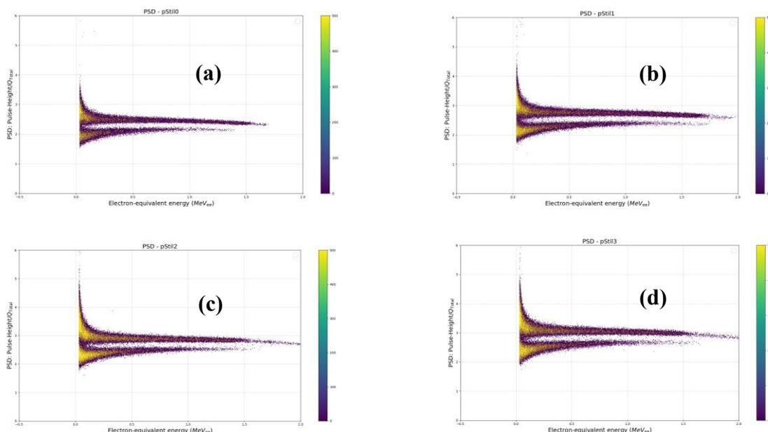
**Figure 4.** 2D PSD histogram for the four stilbene crystals irradiated with a Am-Be source. PSD (Pulse-Height/ $Q_{total}$ ) as a function of electron-equivalent energy (MeV), with a pile-up detection threshold of -300 pC and a low energy threshold of 50 keV. PROTEUS-pStil0 (a), INRAD-pStil1 (b), INRAD-pStil2 (c), INRAD-pStil3 (d).
