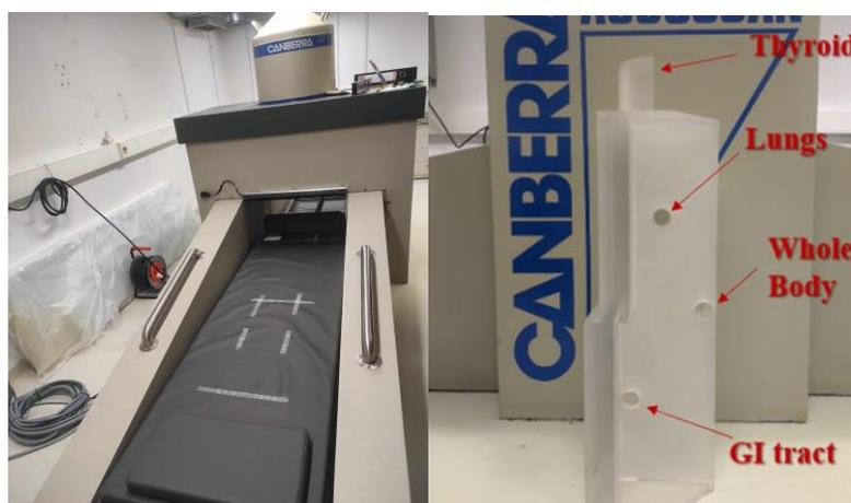
**Figure 1.** (*left*) The Whole body Counter system of EEAE (*right*)The RMC-II phantom
