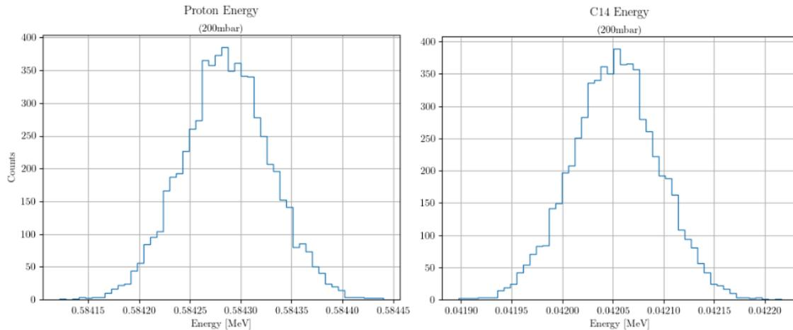
**Figure 7.** Proton (left) and carbon (right) energy at creation for 200 mbar.
