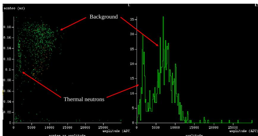
**Figure 10.** Experimental measurements of thermal neutrons for 200 mbar
