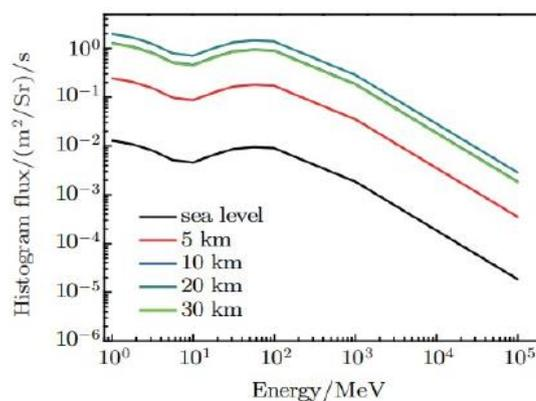
**Figure 2.** Atmospheric neutron spectrum at different altitudes [5]
