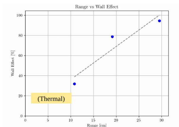
**Figure 4.** Wall effect as a function of particles range for SPC ( $\Phi=30\text{cm}$ ) at 1 bar
