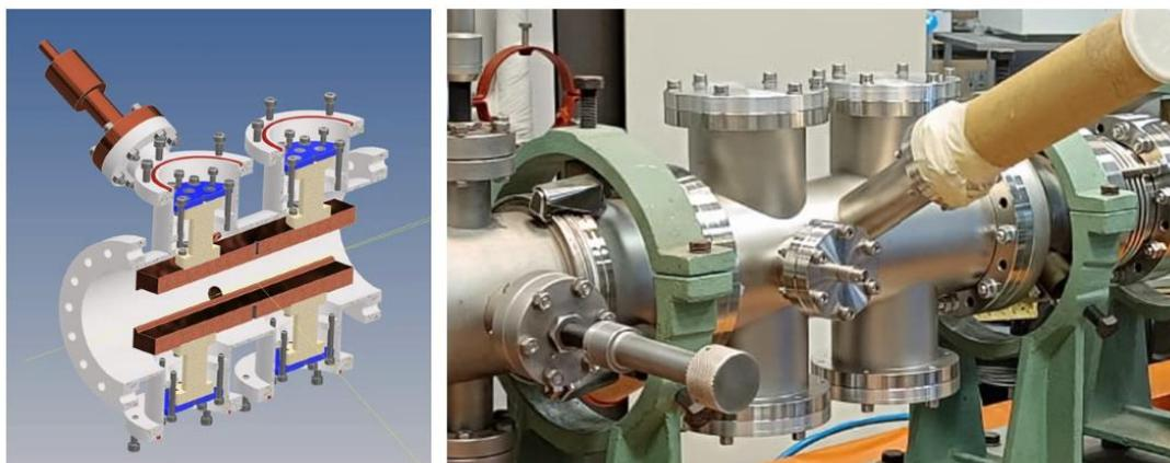
**Figure 3.** Design (left) and implementation (right) of the chopper-buncher system.
