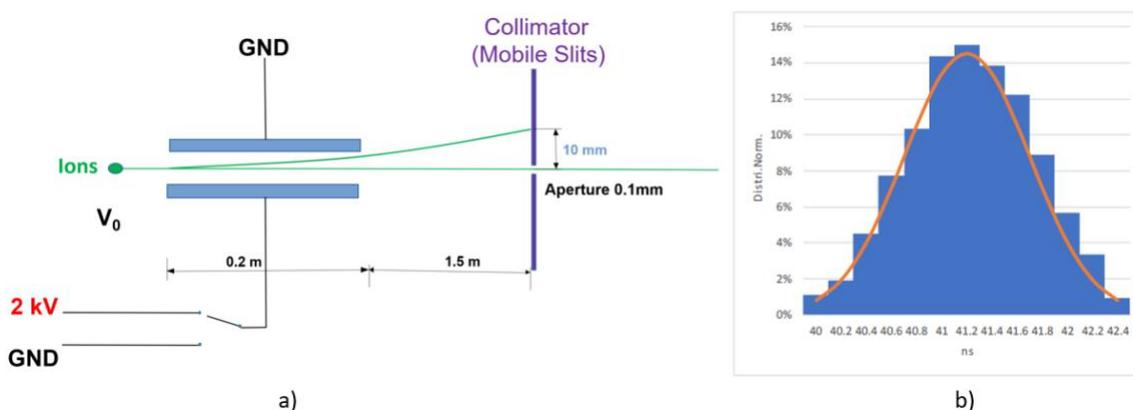
**Figure 2.** Diagram of the chopper-buncher system (a). The deflection of 10 mm and the bunch temporal distribution (b) is obtained with “Opera Simulation Software” for 1 MeV proton beam assuming an electrodes gap of 20 mm.
