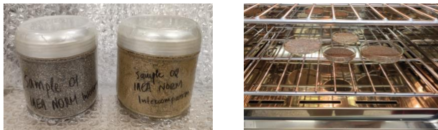
Figure 1. Samples in the containers used (left) and during the drying procedure (right)
