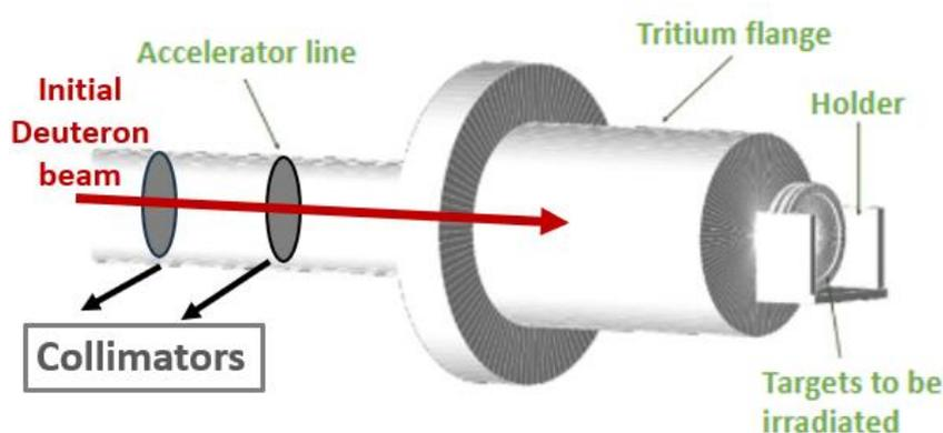
**Figure 6.** Visualization of the geometry of the “Demokritos” experimental setup through the GEANT4 code. The initial deuteron beam is shown in red, then you can see the accelerator line, the two collimators, the tritium flange and the targets to be irradiated, which are on a base (holder).
