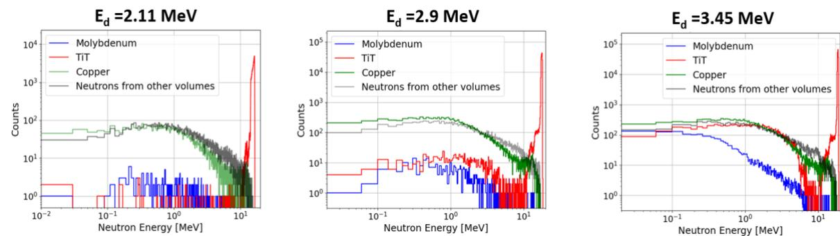
**Figure 8.** Contribution of neutrons from each volume of the total geometry in GEANT4 simulations. The other volumes contributions (black color) are the parasitic neutrons from accelerator line, the collimators, the aluminum flange and the holder.
