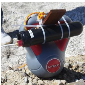
Figure 1. The \gamma Sniffer along with its waterproof housing, during the field measurements in Milos
