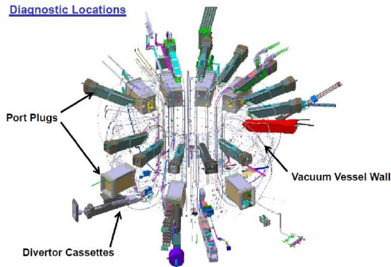
**Figure 1.** *Diagnostics locations at ITER [4]*
