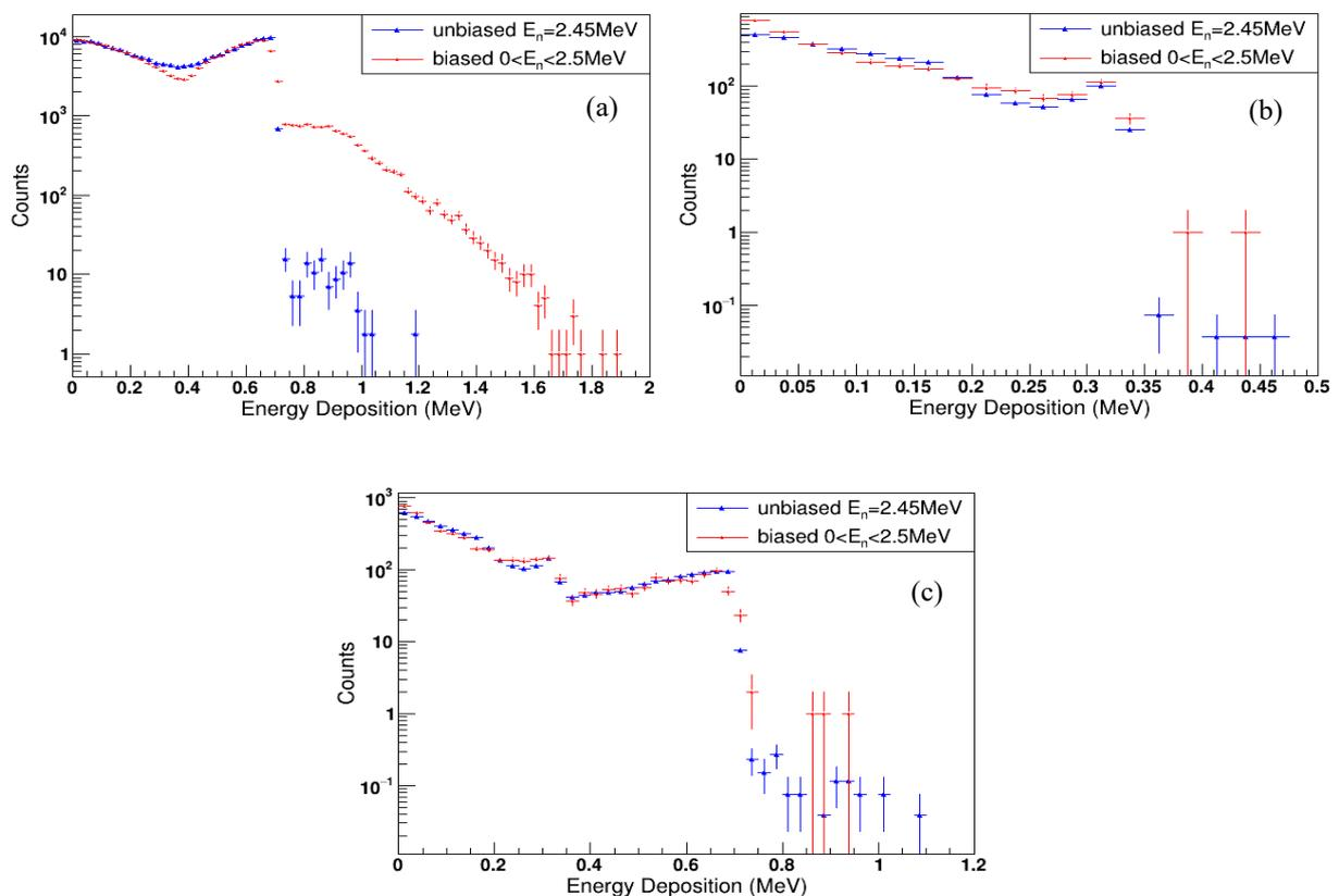
**Figure 5.** Energy deposition spectrum for 2.45 MeV neutrons for a  $50\ \mu\text{m}$  C (a), Si (b) and SiC (c) detector. The blue points derive from a 2.45 MeV monoenergetic neutron beam with  $10^9$  primary neutrons. The red points correspond to  $10^9$  primary protons interacting with the TiT target and producing a variety of neutrons with mean energy of 2.4 MeV.
