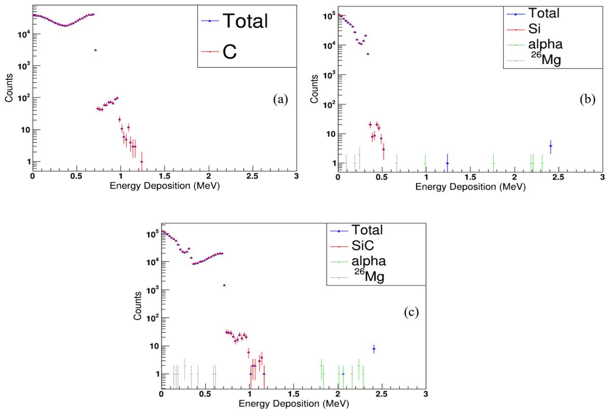
**Figure 2.** Energy deposition spectrum for a 50  $\mu\text{m}$  C (a), Si (b) and SiC (c) detector to 2.45 MeV neutrons. The blue points represent the total energy deposition, the red the corresponding material, the green the alpha particles and the gray the  $^{26}\text{Mg}$  nuclei.
