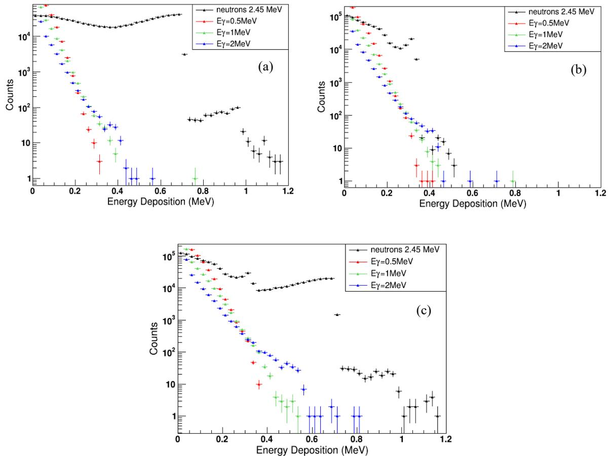
**Figure 3.** Energy deposition spectrum for 500 keV, 1 MeV and 2 MeV  $\gamma$ -rays in a 50  $\mu\text{m}$  C (a), Si (b) and SiC (c) detector. The black points represent the 2.45 MeV neutron energy deposition spectrum.
