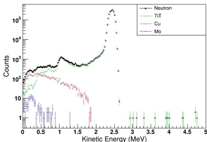
**Figure 4.** Final neutron beam deriving from biasing the TiT target by proton biasing factor=900, with contributions from the Mo and Cu foils
