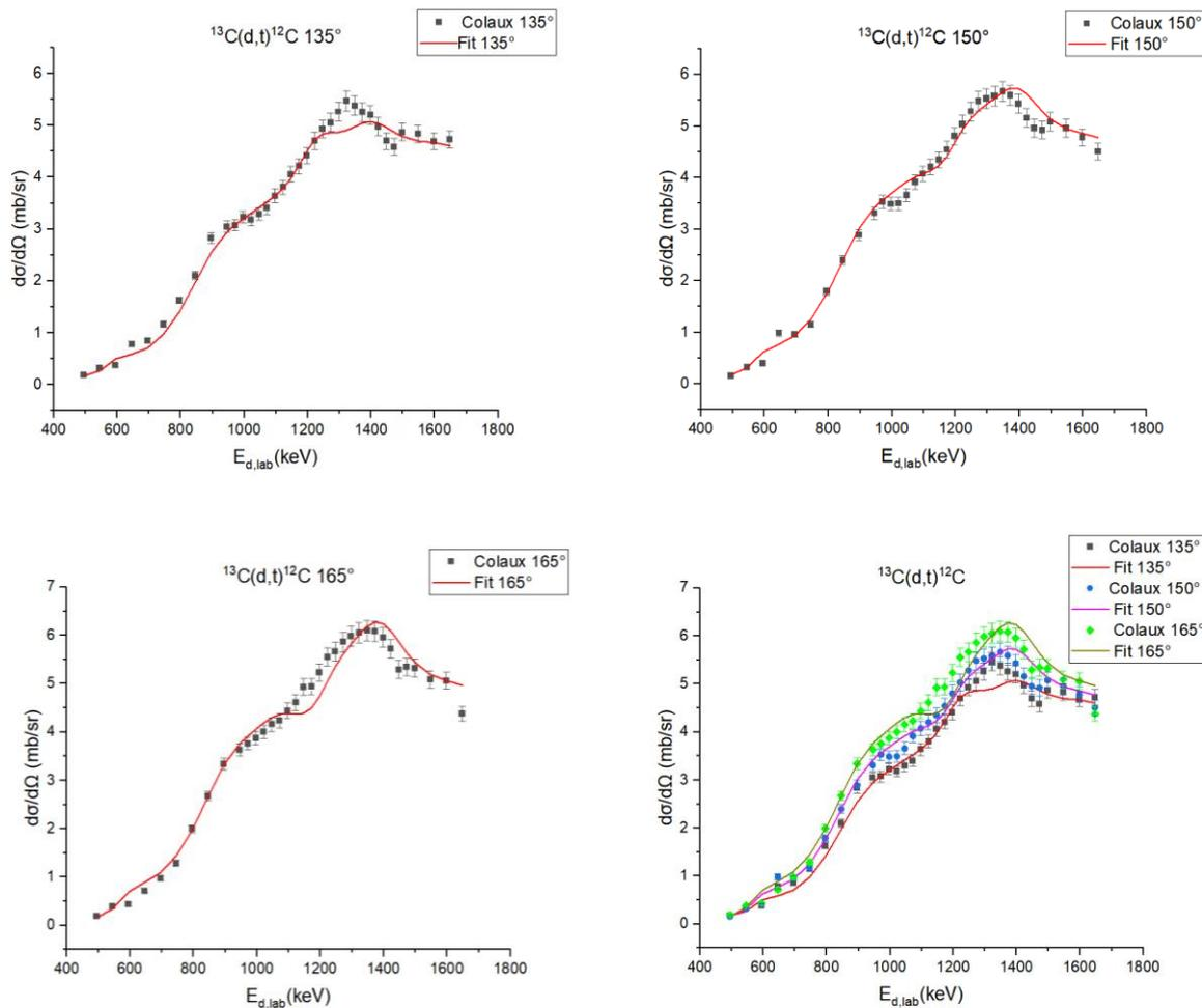
**Figure 2 a – d:** Comparison between the cross sections from the R-Matrix calculations and experimental data for the  $^{13}\text{C}(d,t)^{12}\text{C}$  reaction at a)  $135^\circ$  b)  $150^\circ$  c)  $165^\circ$  and d) all three angles
