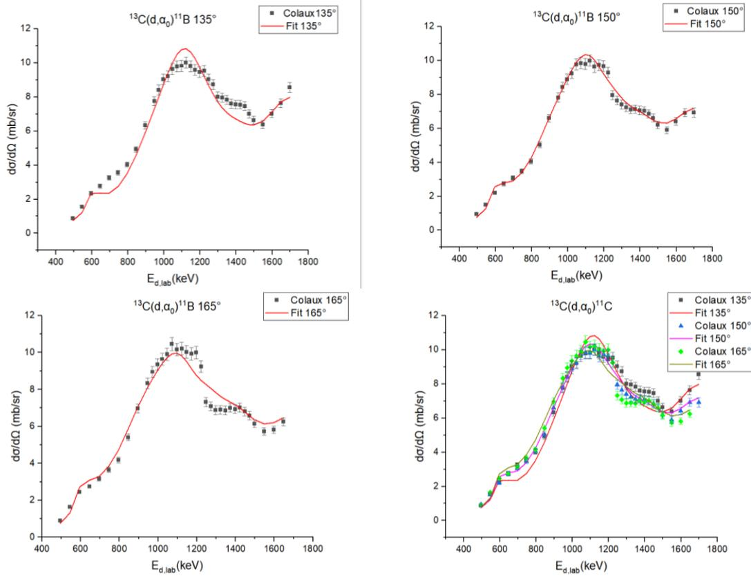
**Figure 3 a – d:** Comparison between the cross sections from the R-Matrix calculations and experimental data for the  $^{13}\text{C}(d, \alpha_0)^{11}\text{B}$  reaction at a)  $135^\circ$  b)  $150^\circ$  c)  $165^\circ$  and d) all three angles
