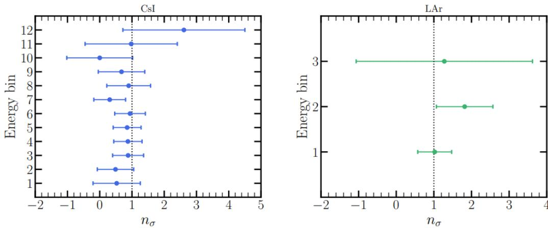
**Figure 2.** Experimentally measured CEvNS cross section normalized to the SM prediction ( $n_\sigma$ ), extracted from COHERENT CsI and LAr data. Results in each recoil energy bin indicate the central value (mean) along with its uncertainty ( $1\sigma$ ) [32].
