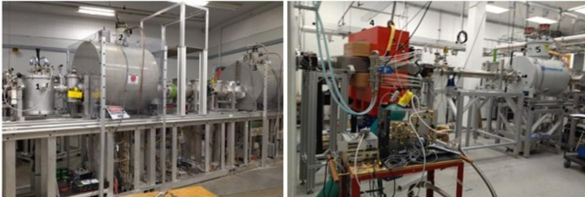
**Figure 2.** Photo of the *TriSol* facility prolonged in two experimental halls. In the first hall we can see the (1) primary gaseous target and the two twin solenoids (2,3). In the adjacent hall the new bending magnet (4) and the third new solenoid (5) before the target chamber, can be also seen.
