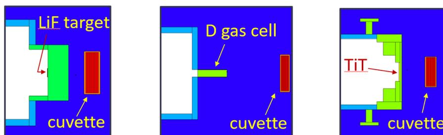
**Figure 1** Representation of the end of the irradiation line along with the flange with the LiF target (left), the deuterium gas cell (middle), the flange with the TiT target (right) and the cuvette which is filled with photosensitizer solution.
