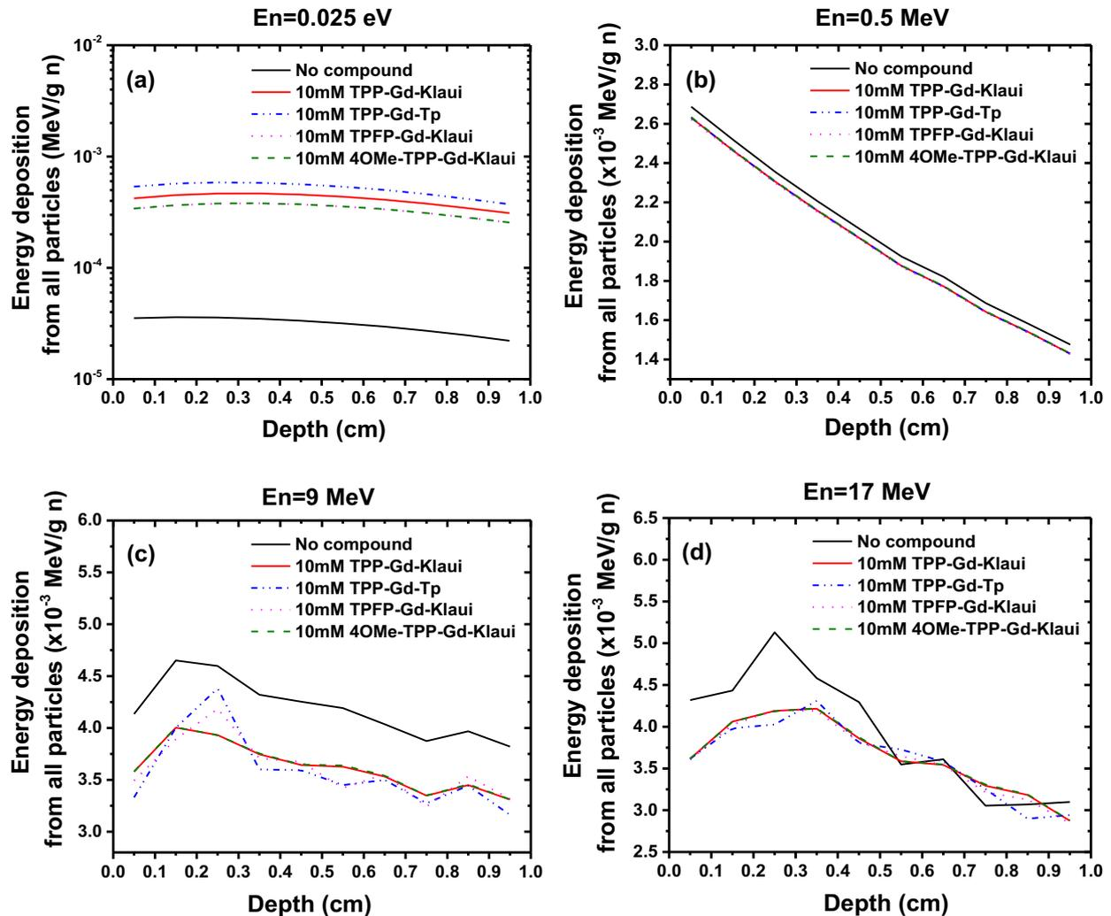
**Figure 3** Energy deposited in the cuvette from all particles in the problem with respect to depth for 0.025 eV, 0.5 MeV, 9 MeV and 17 MeV neutron energies. The statistical errors of the simulations are less than 1%.
