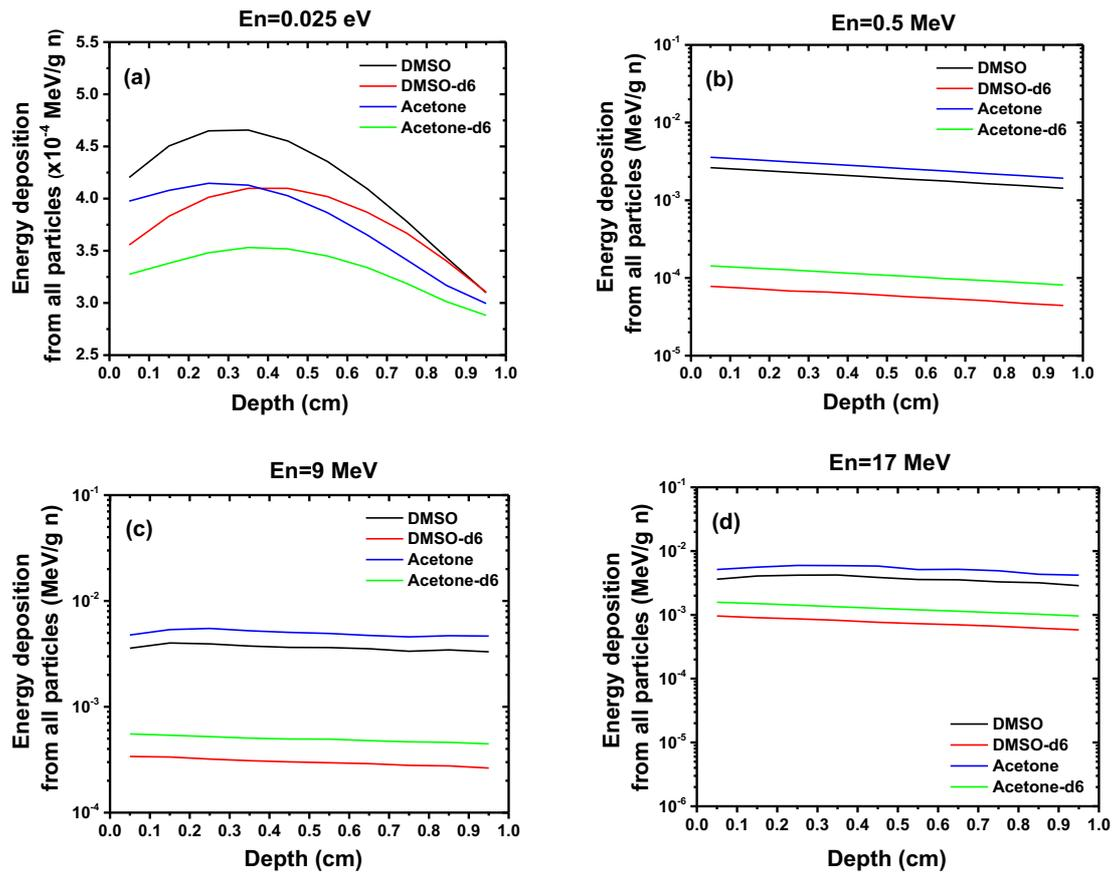
**Figure 4** Energy deposited in the cuvette from all particles in the problem with respect to depth for 0.025 eV, 0.5, 9 and 17 MeV neutron energies, respectively. The statistical errors of the simulations are less than 5%.
