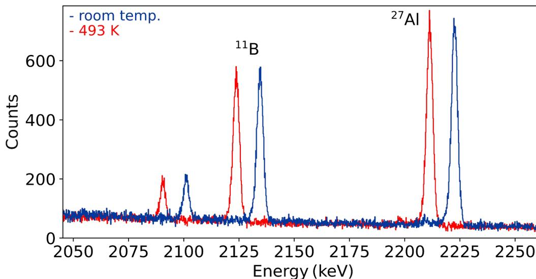
**Fig. 4.** Spectra of the HPGe detector at  $90^\circ$  from the measurement at room temperature (blue) and at 493 K (red). For better visibility, the blue spectrum was shifted to higher energies. The  $^{11}\text{B}$  transition was used to normalize the spectrum from the measurement at room temperature so that the difference in counts for the  $^{27}\text{Al}$  transition is due to self-absorption only. The spectra are the on-line spectra.
