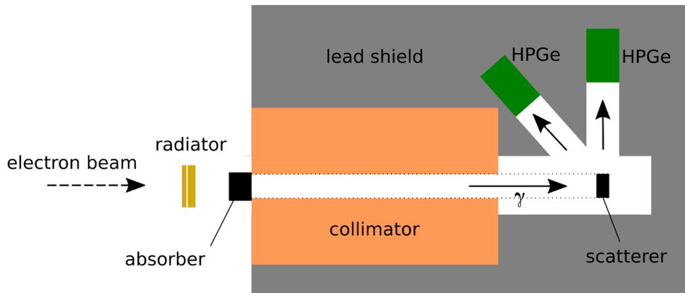
**Fig. 1.** Experimental setup. The absorber was fully covering the collimator opening. As it is shown with the dotted lines, the full size of the scatterer target was irradiated by the photon beam. More details about the setup can be found in the text.
