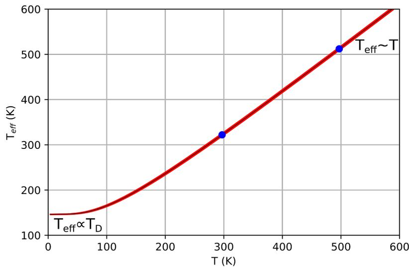
**Fig. 2.** The  $T_{\text{eff}}$  calculated from the Debye theory, equation (3), for  $^{27}\text{Al}$  ( $T_D=390$  K [7]) (black curve). With red the uncertainty band is shown for an uncertainty of 3 K on  $T$ . The two blue dots represent the absorber's temperatures in the experiment performed at DHIPS.
