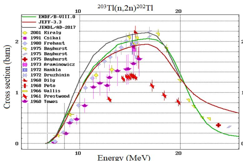
Figure 1: Existing experimental data of  $^{203}\text{Tl}(n,2n)^{202}\text{Tl}$  reaction [4,5].
