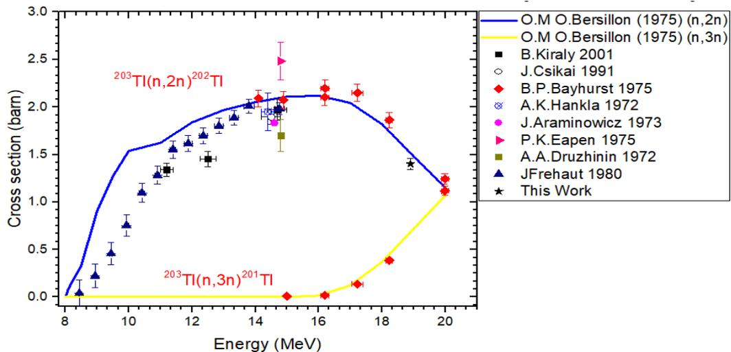
**Figure 5:** The experimental point from the present work along with existing experimental data (since 1970) [5], and EMPIRE code theoretical calculation [8,9].
