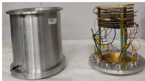
Fig. 1. The aluminum chamber and the target-detector assembly.
