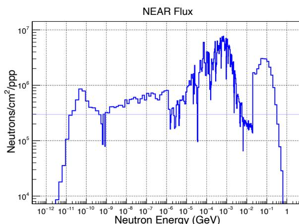
**Figure 2.** The expected neutron flux at NEAR Station.
