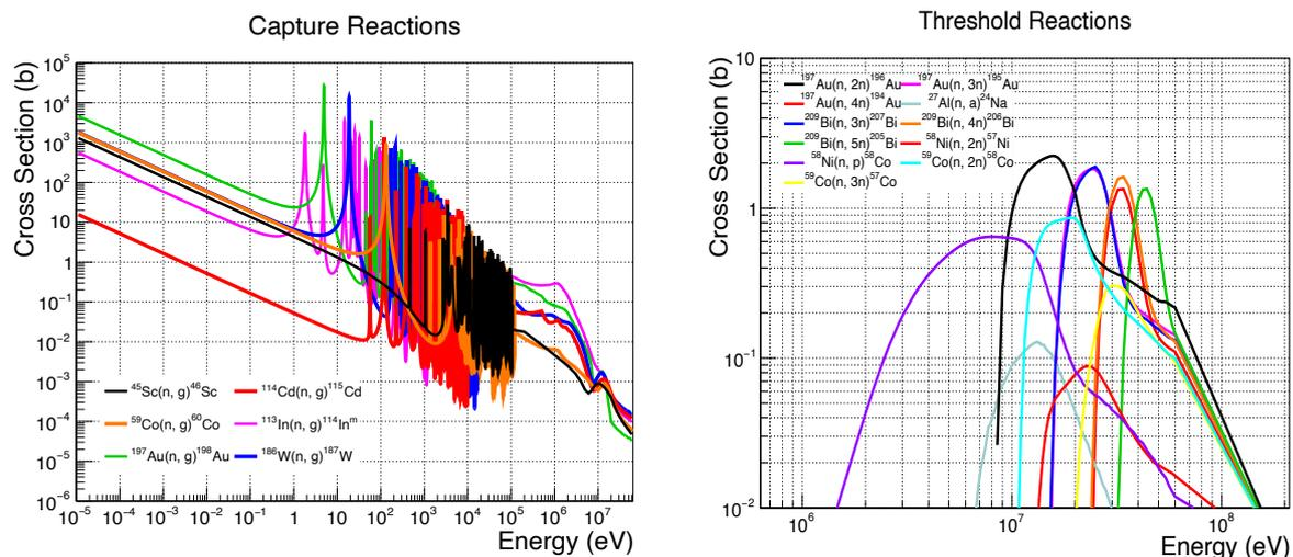
**Figure 1.** Capture cross-sections which were used for the characterization of the neutron flux (left) and the threshold cross sections for the determination of the high neutron energy spectrum (right).
