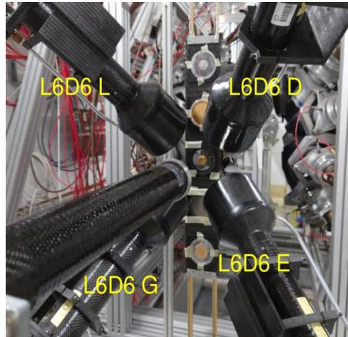
**Fig. 3.** C6D6 liquid scintillators for capture measurements
