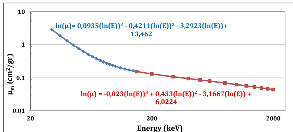
Fig. 3. Mass attenuation coefficient  $\mu_m$  for Lead Slag
