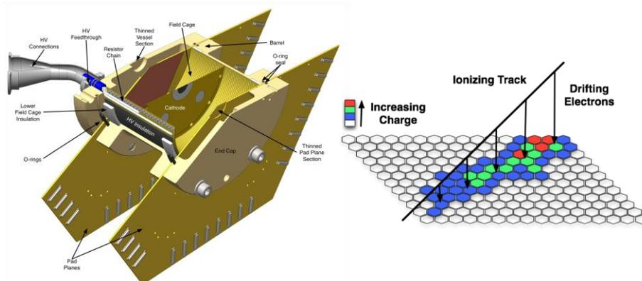
**Fig. 1.** (Left) A cut-away of the fissionTPC detector. Details can be found in Ref. [3]. (Right) A schematic representation of the fissionTPC data reconstruction. Each hexagonal segment of the anode is instrumented and the signal size and time are recorded.
