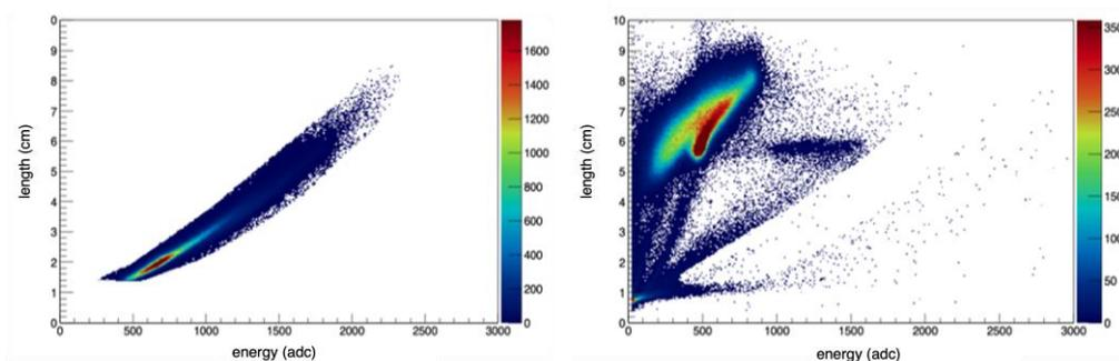
**Fig. 3.** The  $\alpha$ -band selection cut (left) and the corresponding triton tracks (right) that also pass the shared vertex and angular selections. Background reactions from alternative  ${}^6\text{Li}+n$  reaction channels and beam-induced accidental coincidences can also be seen, particularly at lower energies.
