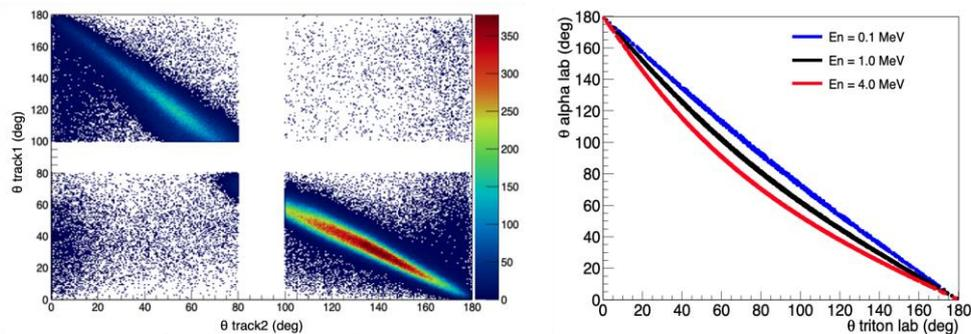
**Fig. 4.** (Left) The angular correlation for the  ${}^6\text{Li}(n,t)\alpha$  events in the data for a range of neutron energies. The empty regions in the center of the angular range is due to an additional angular selection cut. (Right) The angular correlation between the particles in the  ${}^6\text{Li}(n,t)\alpha$  determined by a kinematics calculation for single incident neutron energies.
