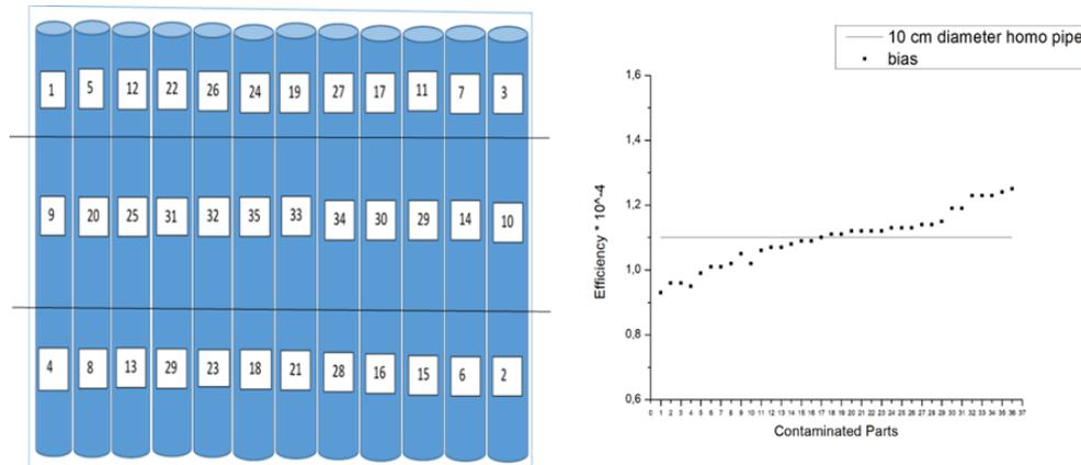
**Fig. 4.** On the left is the configuration of the 10 cm diameter pipes in the 1.2m x 1.2m shallow box where the segments of the pipes are also shown. On the right the total efficiency for homogeneous activity distribution on the pipes (line) as well as the efficiency of each segment (points) are presented.
