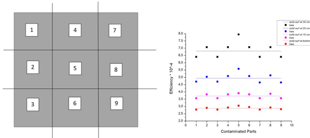
**Fig. 5.** On the left is the metallic slab 0.6m x 0.6m x 0.005m divided into 9 segments. On the right the total efficiency for homogeneous activity distribution inside the slab (lines) as well as the efficiency of each segment (points) are presented
