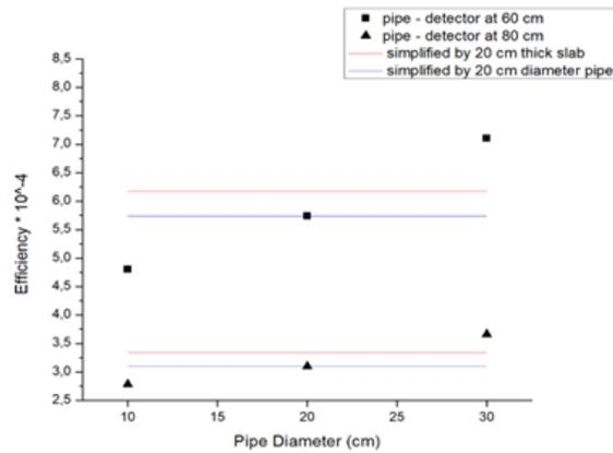
Fig. 6. Efficiencies of pipes and simplified geometries
