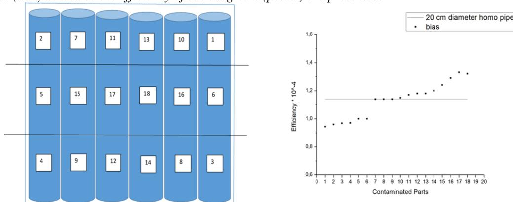
**Fig. 3.** On the left is the configuration of the 20 cm diameter pipes in the 1.2m x 1.2m shallow box, where the segments of the pipes are also shown. On the right the total efficiency for homogeneous activity distribution on the pipes (line) as well as the efficiency of each segment (points) are presented.
