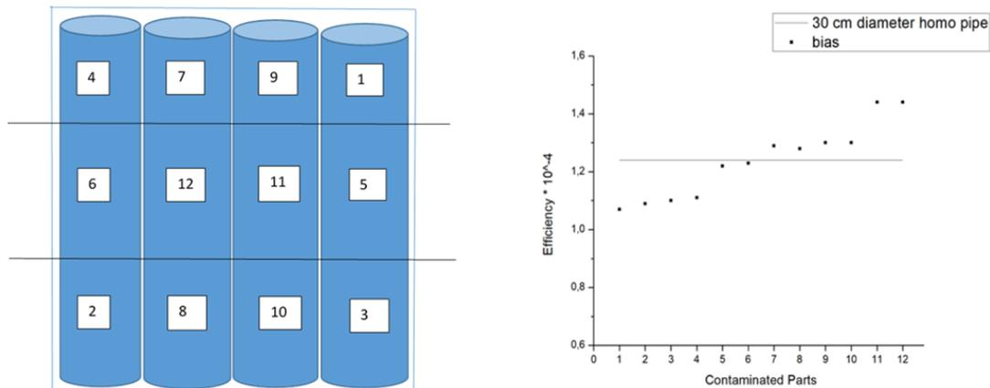
**Fig. 2.** On the left is the configuration of the 30 cm diameter pipes in the 1.2m x 1.2m shallow box where the segments of the pipes are also shown. On the right the total efficiency for homogeneous activity distribution on the pipes (line) as well as the efficiency of each segment (points) are presented.
