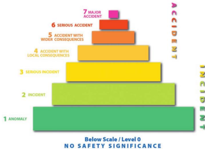
Fig. 1. Schematic of the 7 levels rating of the nuclear and radiological events. The events are classified in accidents and incidents [4] (Reproducing with permission by IAEA).
