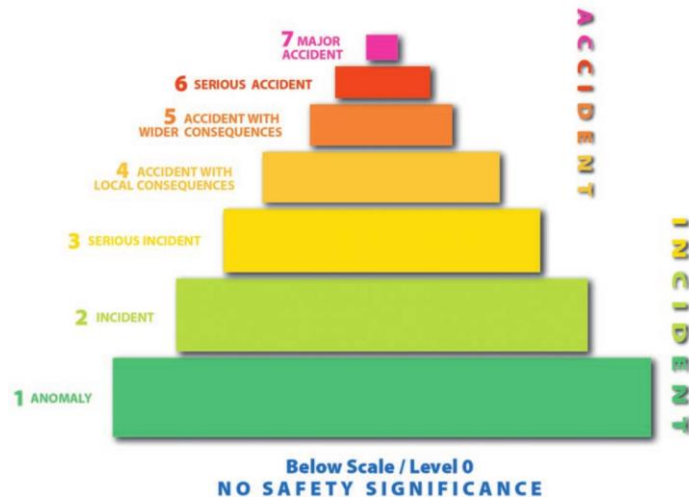
Fig. 1. Schematic of the 7 levels rating of the nuclear and radiological events. The events are classified in accidents and incidents [4] (Reproducing with permission by IAEA).
