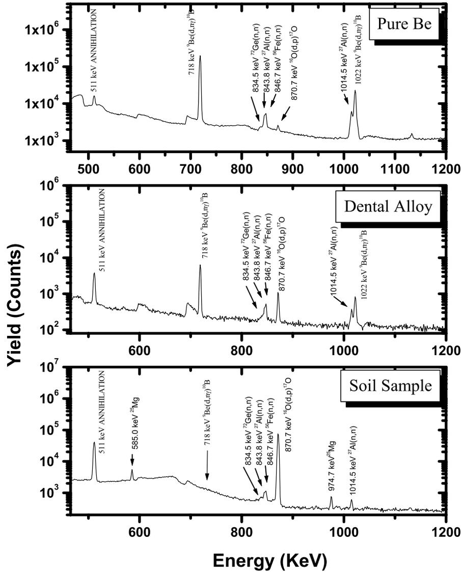
Figure 4: Spectra taken from the (d,n $\gamma$ ) reaction taken at 1.5 MeV deuteron beam energy, for 20 $\mu\text{Cb}$  accumulated charge. a) Metallic Be target, b) dental alloy c) Typical soil sample
