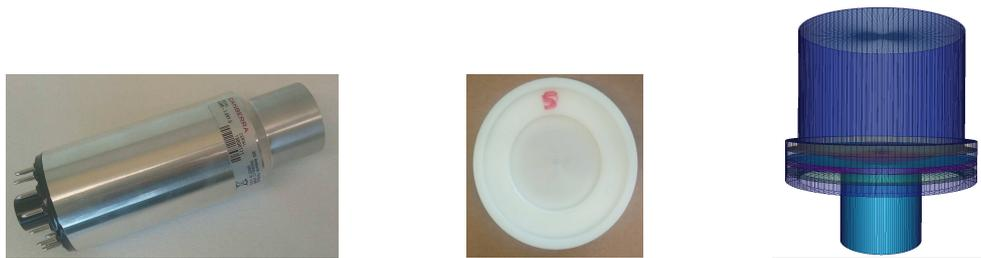
**Fig. 1.** The LaBr<sub>3</sub>(Ce) detector, the acetal holder and the MCNP-X simulation of the gamma volume source (from left to right)
