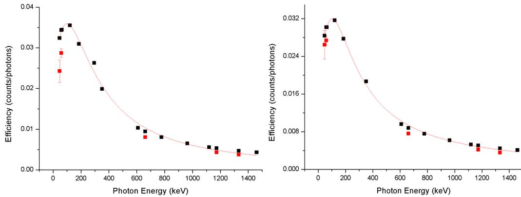
**Fig. 3.** Efficiency calibration curves for the 0.5 g/cm<sup>3</sup>(left) and 0.9 g/cm<sup>3</sup>(right) volume source
