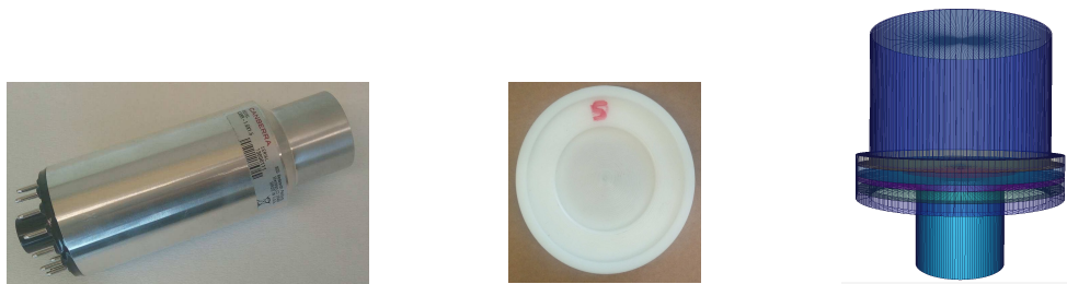
Fig. 1. The LaBr 3 (Ce) detector, the acetal holder and the MCNP-X simulation of the gamma volume source (from left to right)
