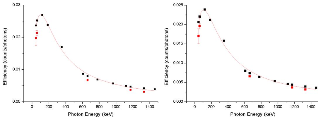
**Fig. 4.** Efficiency calibration curves for the 1.5 g/cm<sup>3</sup>(left) and 2.0 g/cm<sup>3</sup>(right) volume source
