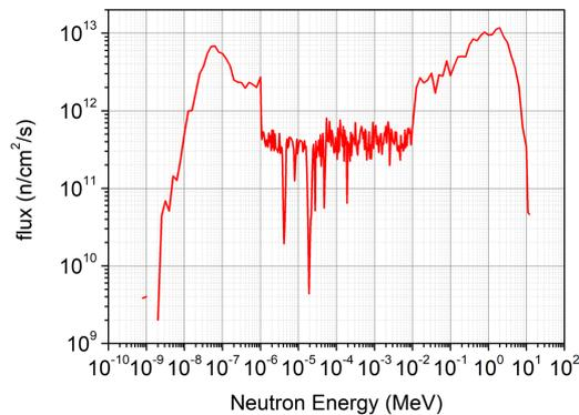
**Figure 2.** Neutron spectrum at position G180 channel of BR2 (where the samples were irradiated), used for FISPACT-II calculations.
