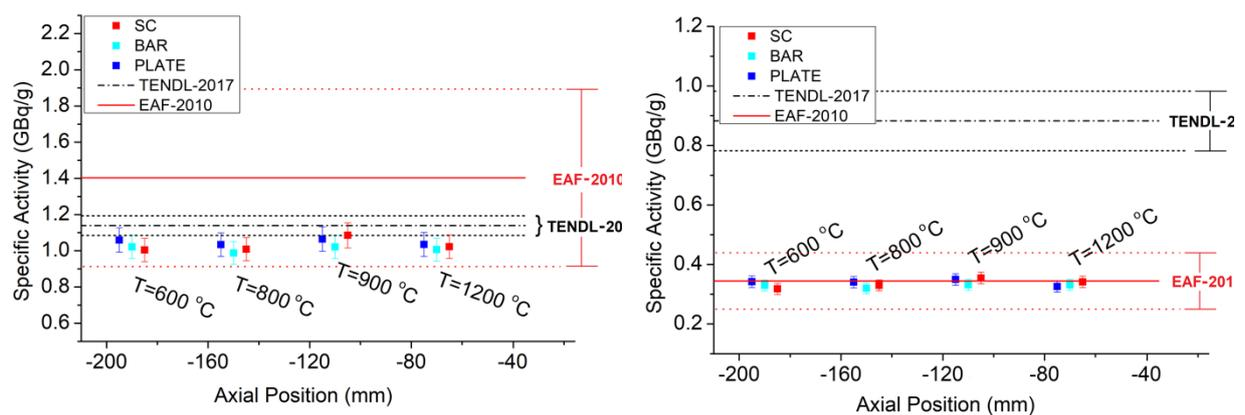
**Figure 4.** Specific activity of  $^{185}\text{W}$  (left) and  $^{181}\text{W}$  (right) for 0.18 dpa samples normalized to 0.2 dpa, at 475 days after the end of irradiation, versus axial position in the irradiation channel.
