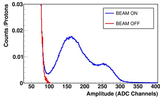
**Figure 3.** An example of beam-on (blue) and beam-off (red) pulse height spectrum for one of the  $^{241}\text{Am}$  targets. As can be seen, the alpha-decay particles are well separated from the fission fragments but still an amplitude threshold has to be applied in the analysis along with the corresponding correction factor.
