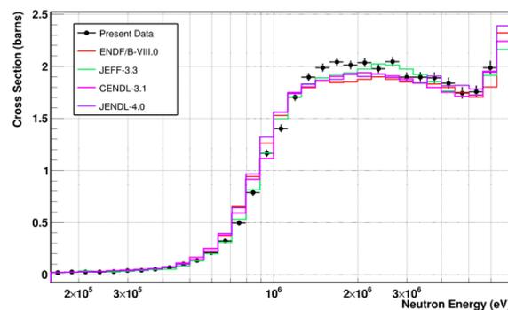
**Figure 5.** Preliminary  $^{241}\text{Am}(n,f)$  cross section derived from the weighted average from the americium samples. The error bars represent the statistical uncertainty. The experimental data are normalized to the evaluated libraries at 1.2 MeV for comparison.
