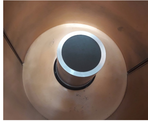
Figure 2. Depiction of the BE5030 HPGe detector
