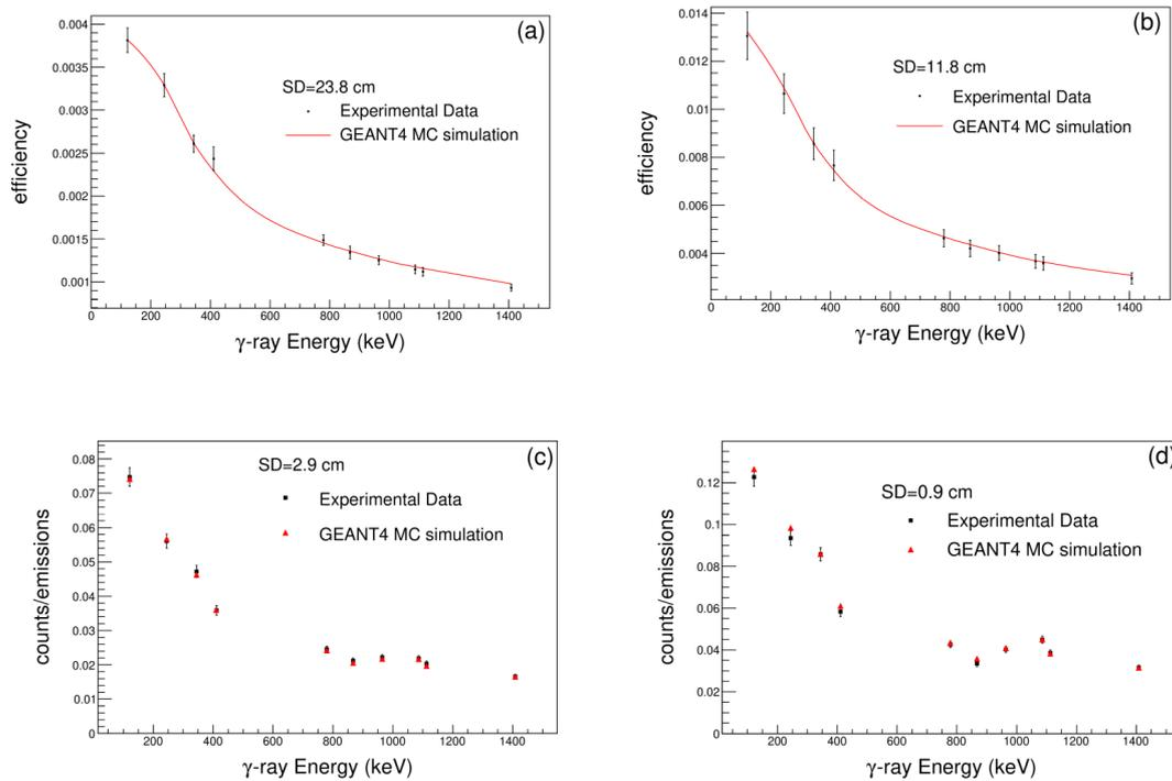
**Figure 2:** Comparison of the experimental efficiency and counting rate data of the 80% relative efficiency HPGe detector with the GEANT4 MC code simulations at the distances of (a) 23.8 cm (b) 11.8 cm (c) 2.9 cm (d) 0.9 cm with respect to the detector window.
