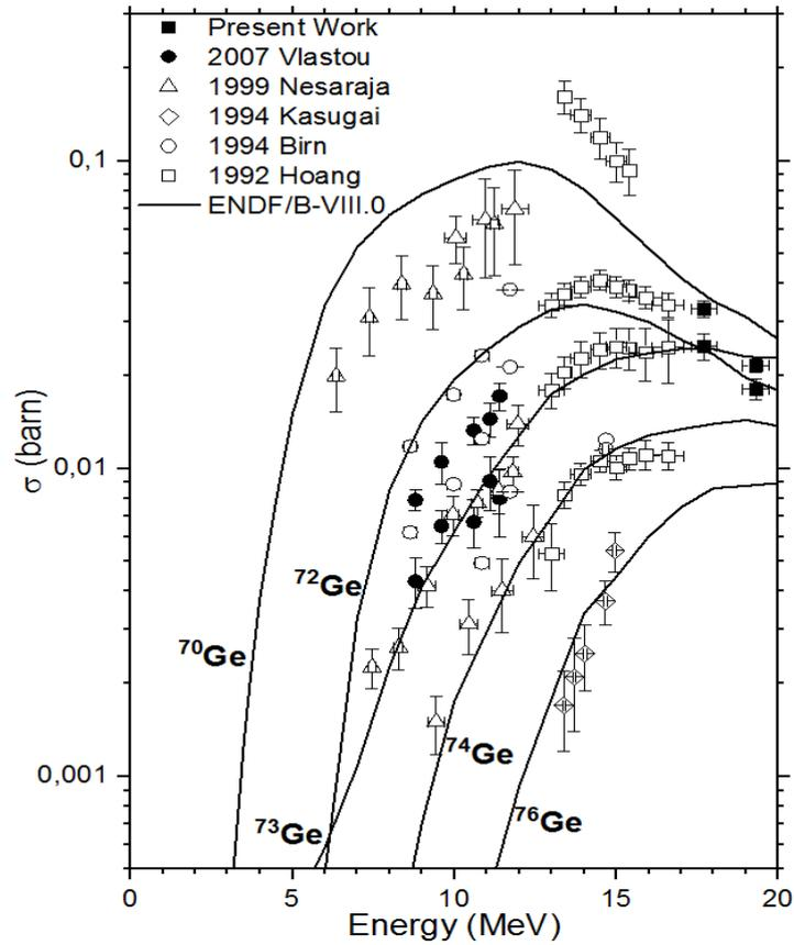
**Figure 3.** Cross-section data of the  $(n,p)$  reactions on Ge isotopes along with ENDF values (solid line). The black squares are the data of the present work, while the black circles are the data from previous work of our group [2].
