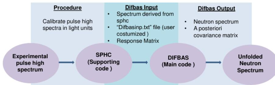
Figure 2. Flowchart of unfolding procedure and DIFBAS code
