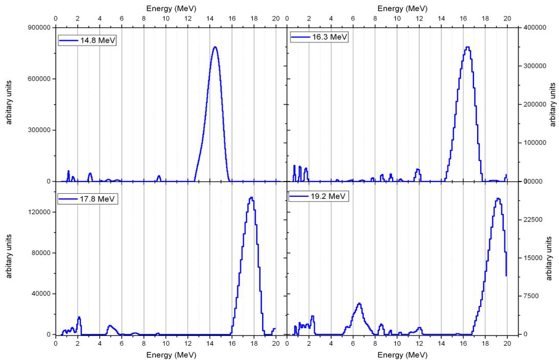
Figure 5. Deconvoluted neutron spectra using DIFBAS code
