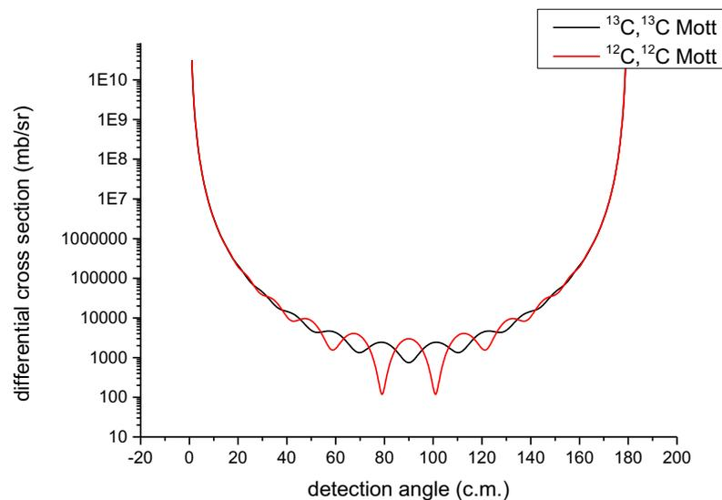
**Figure 2.** Angular distribution of the Mott scattering differential cross section of  $^{13}\text{C}$  (black) with a spin  $\frac{1}{2}$  and of  $^{12}\text{C}$  (red) with a spin 0 in the Center of Mass reference frame for  $K = 3 \text{ MeV}$ .
