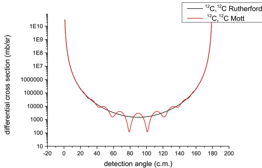
**Figure 1.** Angular distribution of the differential cross section of the elastic Mott Scattering (red) and the expected Rutherford values (black) of  $^{12}\text{C}$  for  $K = 3 \text{ MeV}$  in the Center of Mass Reference frame.
