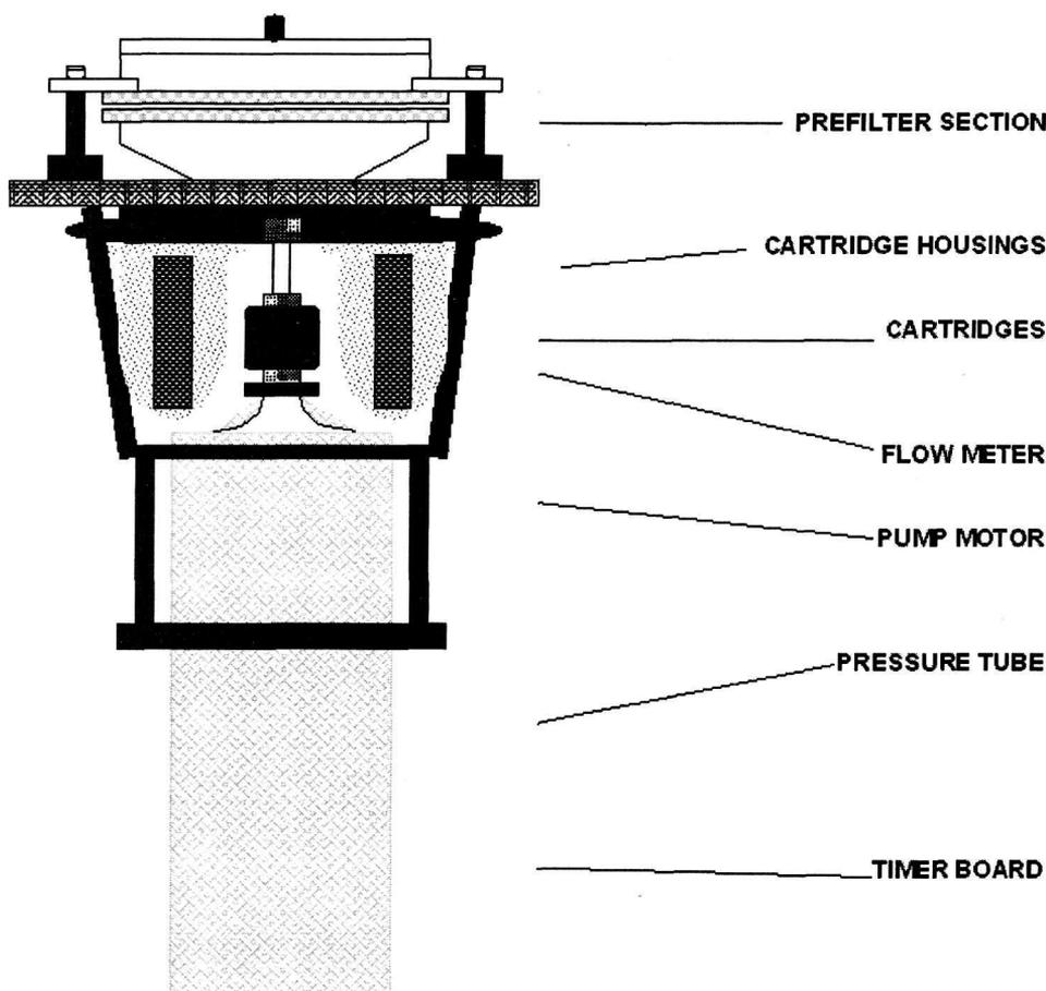
Fig. 2. Main Units of Mark III Centrifugal Pump
