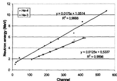
Fig. 4. Energy Calibration of He-3 and He-4 (recoil peak) proportional counter
