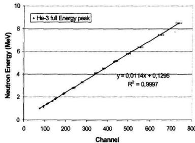
Fig. 3. Energy Calibration of He-3 proportional counter.
