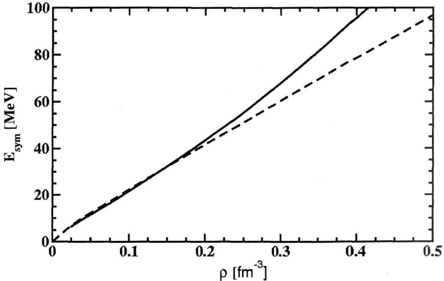
Fig. 5. Density dependence of the symmetry energy  $E_{\text{sym}}$  using only the  $\rho$ -meson field (dashed curve) and both, the  $\rho$ - and  $\delta$ -meson fields (solid curve), taken from [5,12].
