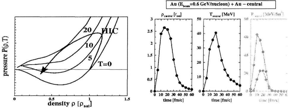
Fig. 2. Phase diagram of nuclear matter at different temperatures (as indicated) and trajectory of nuclear matter through the phase diagram in a HIC. (Right) Time evolution of the local density (left), the local temperature (middle) and the longitudinal (solid) and transversal (dashed) pressures (right) in a central Au on Au collision at 0.6 AGeV bombarding energy per nucleon.
