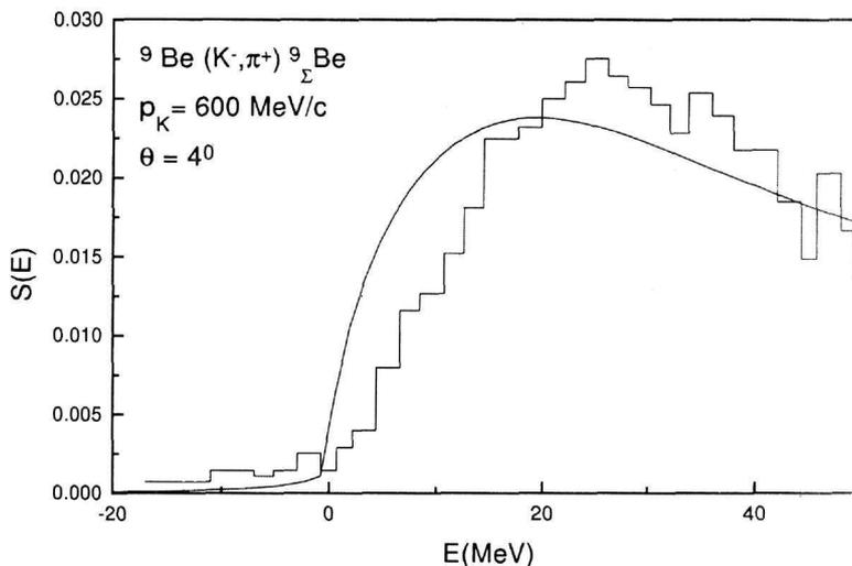
Fig. 4. The calculated spectrum for  $V_c = (50, -i15) \text{ MeV}$  and  $V_{so} = 15 \text{ MeV}$  for the in-flight BNL experiment for  ${}^9_{\Sigma}\text{Be}(K^-, \pi^+)$  and  $\theta = 4^\circ$  together with the experimental spectrum of ref. [2].
