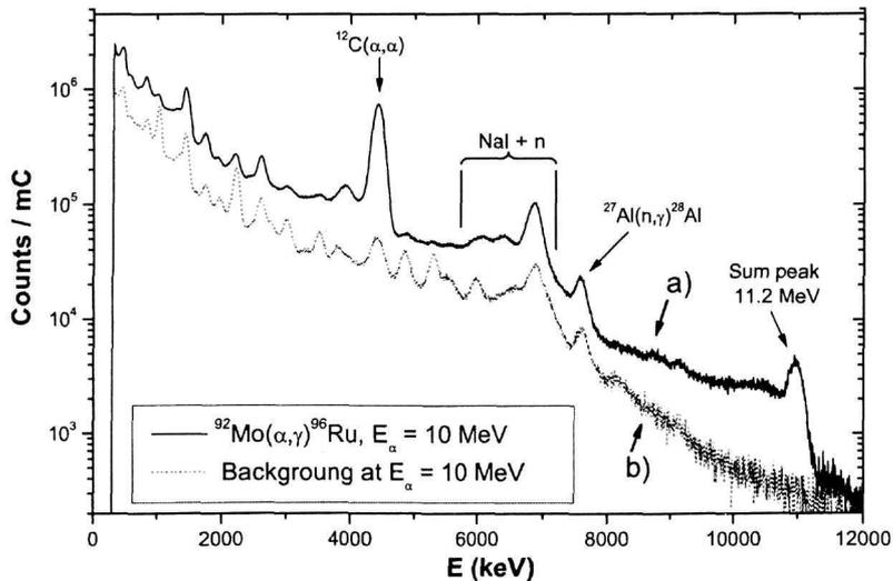
Fig. 1. a) Gamma spectrum of the  $^{92}\text{Mo}(\alpha,\gamma)^{96}\text{Ru}$  reaction taken at  $E_\alpha = 10$  MeV. b) Beam induced background spectrum at the same beam energy.
