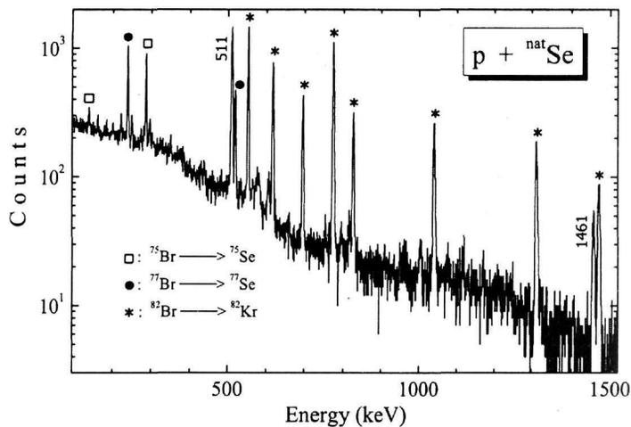
Fig. 2. Activation spectrum measured at  $E_p=5$  MeV for the  $p + {}^{\text{nat}}\text{Se}$  reaction.
