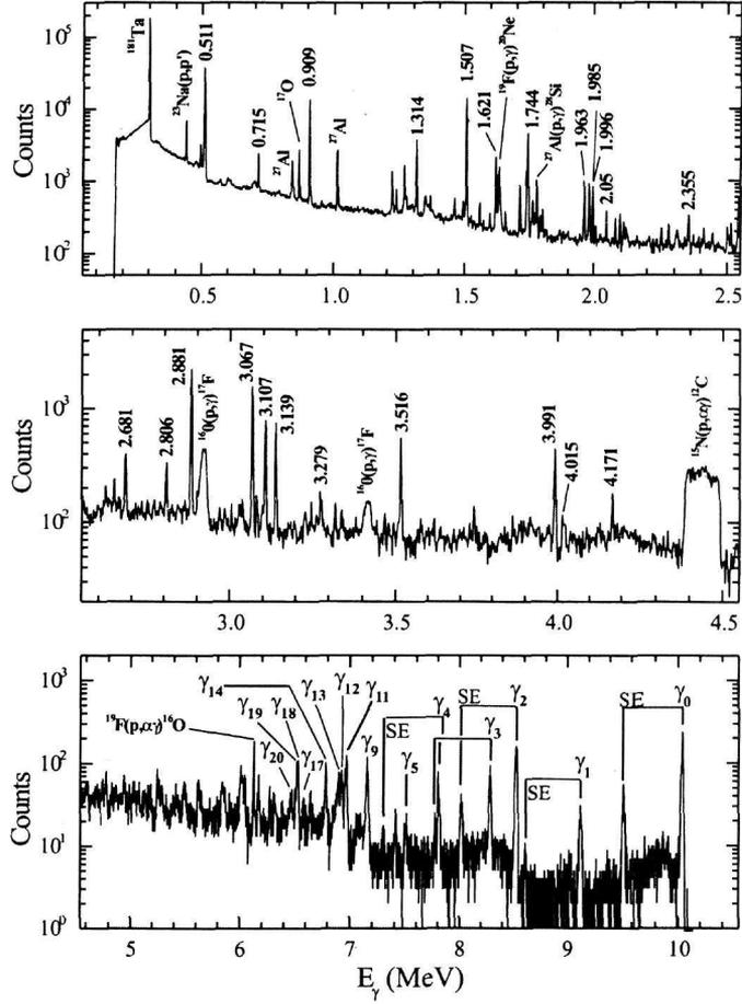
Fig. 2. Typical spectrum of the  $^{88}\text{Sr}(p,\gamma)^{89}\text{Y}$  reaction taken at the energy of 3 MeV, at  $90^\circ$  with respect to the beam direction. The  $\gamma$  transitions relevant to the determination of the cross section are labeled by their energy. In addition to these the  $\gamma_0$  transition at  $\approx 10$  MeV was taken also into account.
