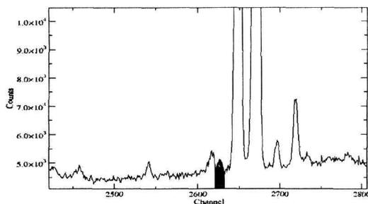
Fig. 1. An enlarged view of the  $\gamma$  ray spectrum of the  $^{241}\text{Am}$  target, at the area of interest for the activation measurement. The shaded peak corresponds to the 987.76 keV transition from the deexcitation of  $^{240}\text{Am}$ , to  $^{240}\text{Pu}$ . All the other peaks observed, are characteristic  $\gamma$  rays from  $^{154}\text{Eu}$  contained in the target.
