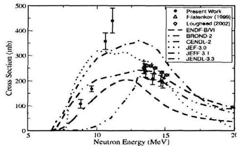
Fig. 4. The cross section of  $^{241}\text{Am}(n, 2n)$  reaction in comparison with recent evaluations and previous measurements [3,4]
