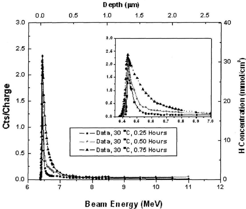
Fig. 1. Examples of hydrogen depth profiles in cement
